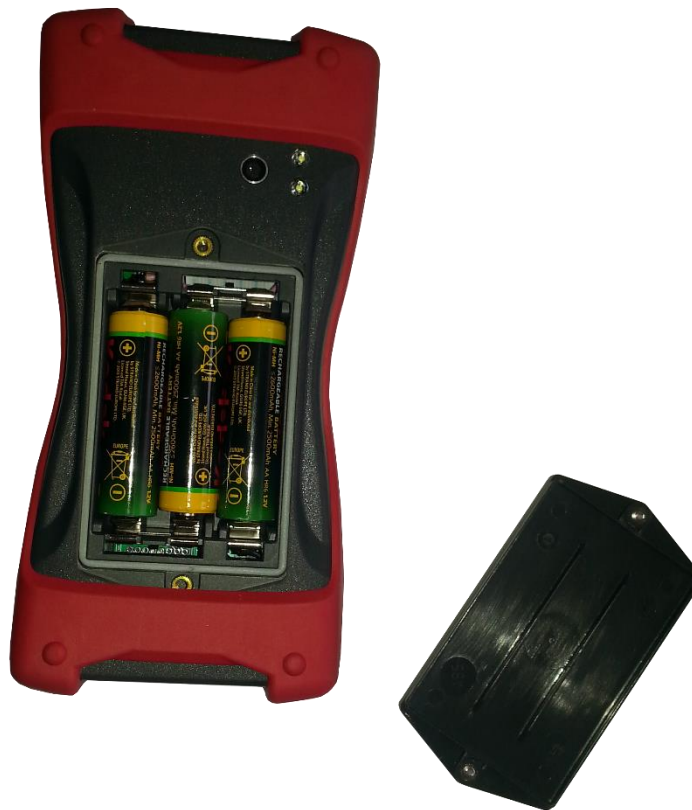
Figure 2.1 - Installing the batteries
