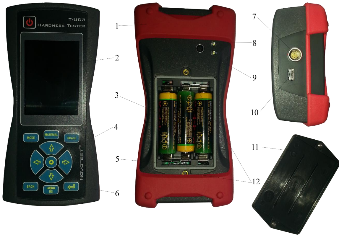
1 – bumper; 2 – LCD/TFT color contrast display; 3 – NiMH battery; 4 – control keyboard; 5 – battery compartment; 6 – electronic unit; 7 – probe socket; 8 – flash light; 9 – photo camera; 10 – mini USB socket; 11 – cover; 12 – cover securing with threaded connections.
